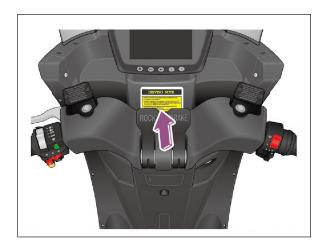
◆ The parking brake warning is located under the parking brake lever.
