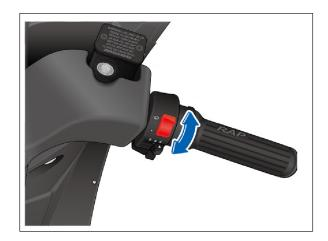
With the ignition switch at "ON", if the windshield washer button is pressed long, the windshield washer will spray water and the wiper also start to operate.
