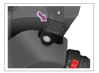
◆ The driving warning is located under the combination instrument.
