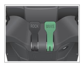
handle is pulled up. When releasing the parking brake, hold the hand brake tightly and then put down the parking handle.
